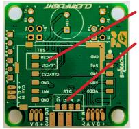
TBS Unify Pro: Install ONE peice of Polyimide tape over the 2 pads in the box labelled `TBS`.
